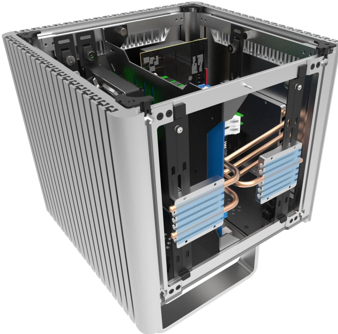
**Warning!** Make sure you peel away the protective flim on both sides of the thermal pad
