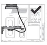
If your configuration requires to have the radiator located below the water pump, you need to ensure that the tubing part of the radiator is located at the bottom while installed. Hissing or Bubbling noise will take longer to disappear than if the radiator is above the card but will ultimately disappear.
